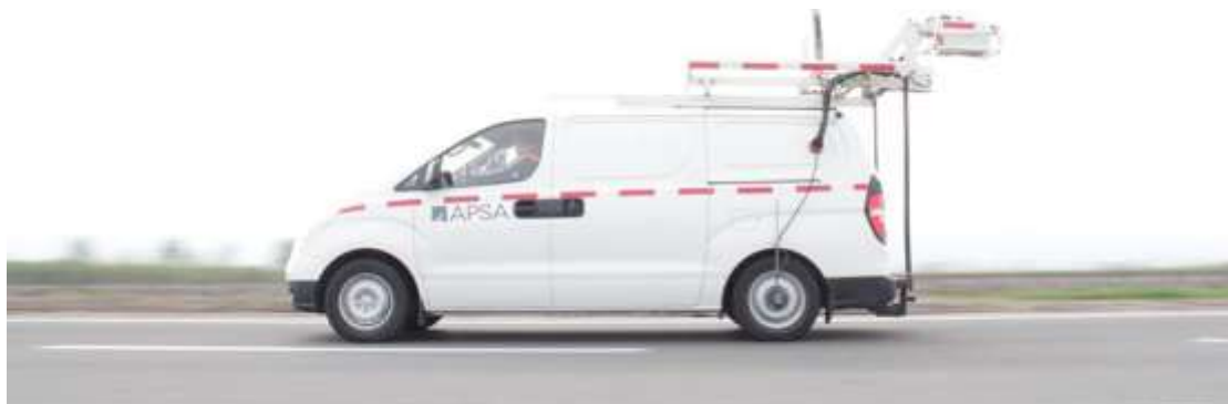
Figura 19: Equipamento Laser Crack Measurement System .
